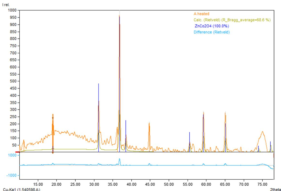
**Fig. 2.** XRD pattern with Rietveld refinement of ZnCo<sub>2</sub>O<sub>4</sub>.
