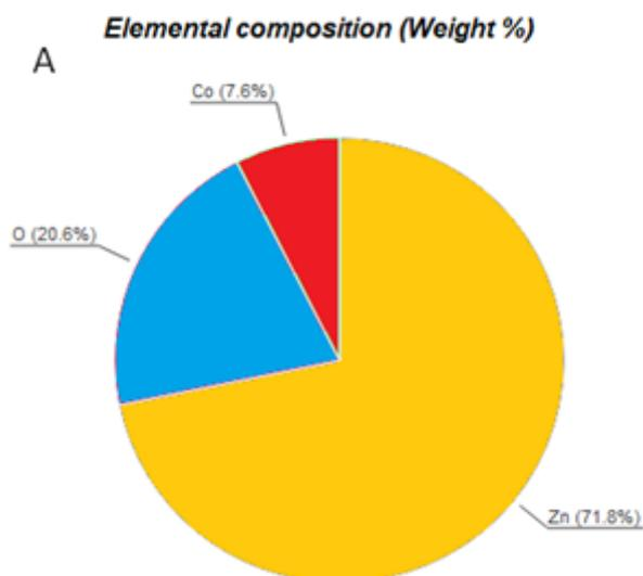
**Fig. 6 (A) Elemental weight percent of Zn/ZnCo<sub>2</sub>O<sub>4</sub> calculated by Rietveld refinement**
