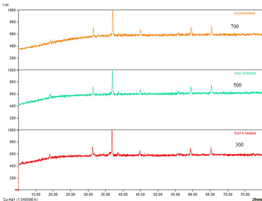
Fig. 1. XRD pattern of ZnCo<sub>2</sub>O<sub>4</sub>.
