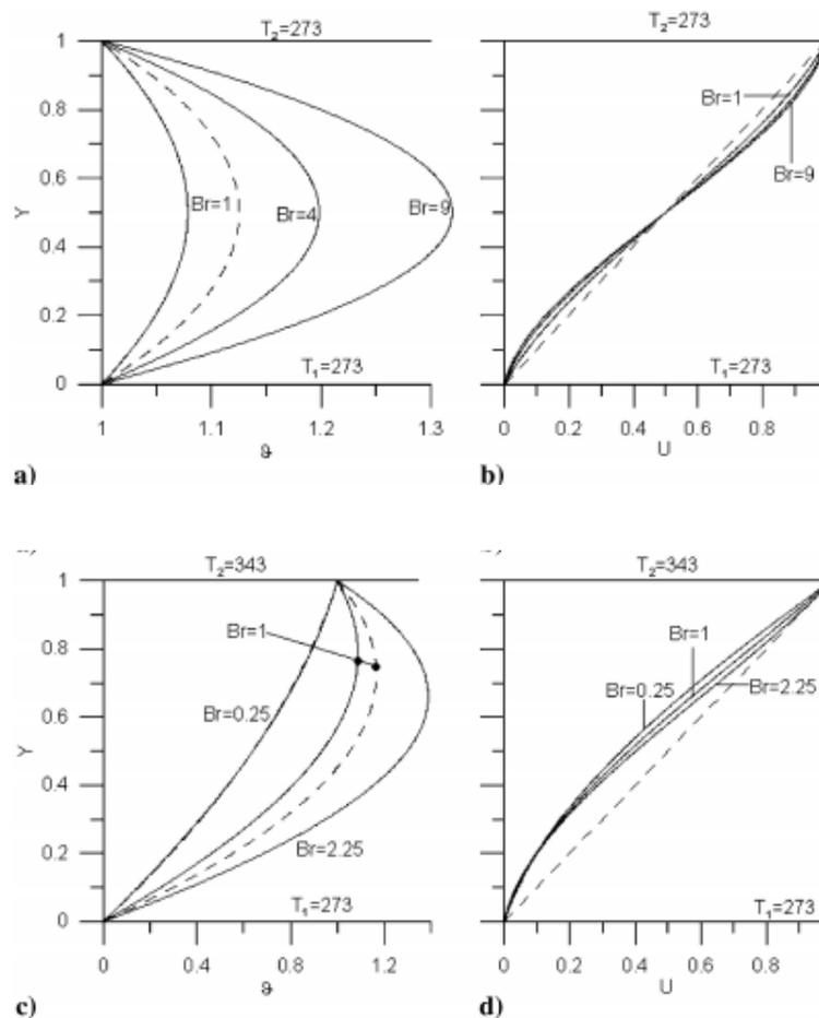
**Fig. 5** Temperature and velocity distribution for water [solid line, present work with variable properties; dashed line, solution for a fluid with constant properties (analytical solution)].
