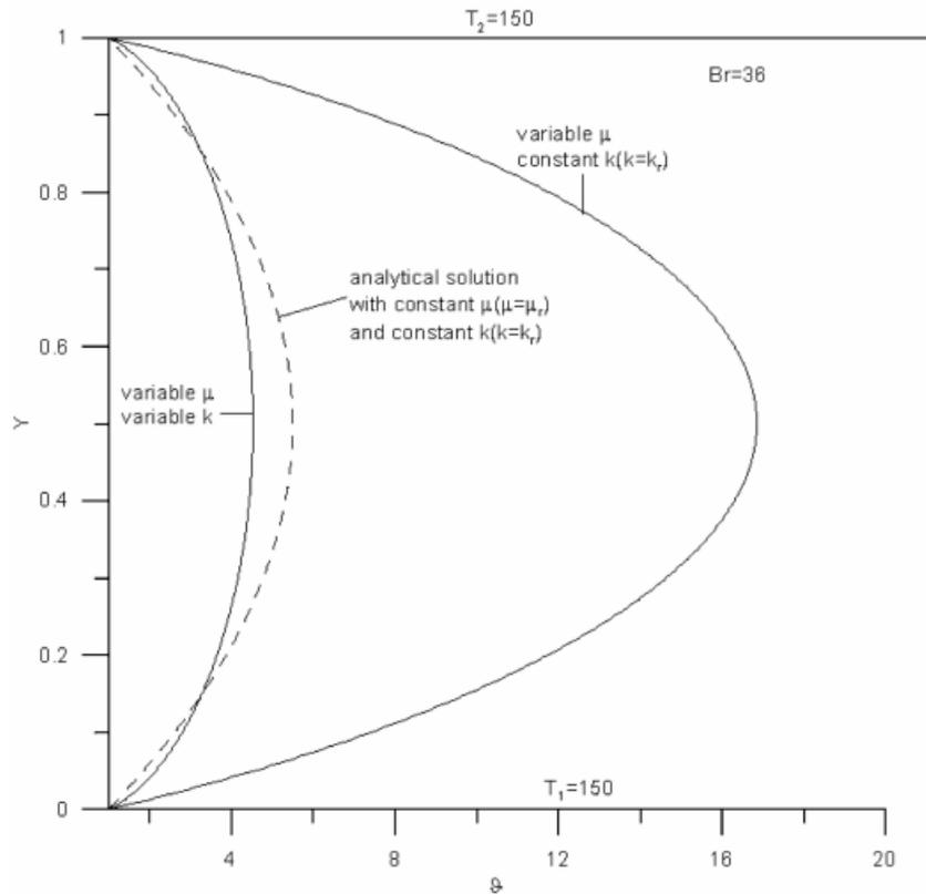
**Fig. 1 Influence of air viscosity and thermal conductivity on the temperature profile for  $Br = 36$  (solid line, present work; dashed line, analytical solution).**
