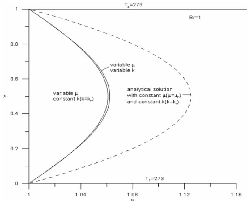
**Fig. 3 Influence of oil viscosity and thermal conductivity on the temperature profile for  $Br = 1$  (solid line, present work; dashed line, analytical solution).**
