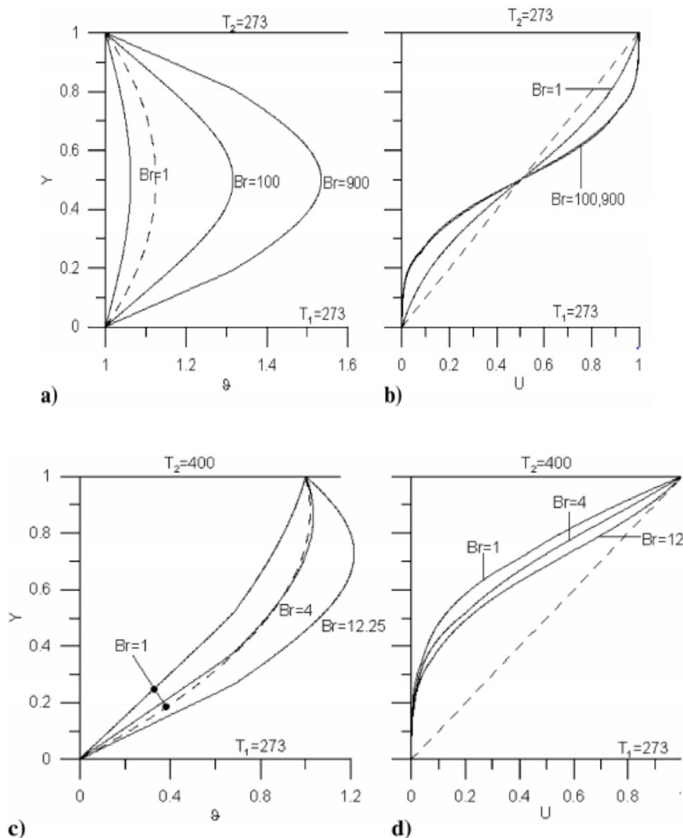
**Fig. 4** Temperature and velocity distribution for oil [solid line, present work with variable properties; dashed line, solution for a fluid with constant properties (analytical solution)].
