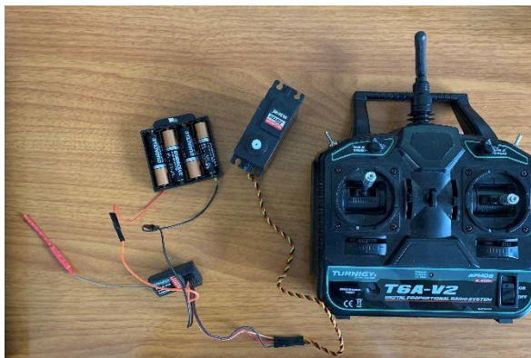
Figure 2: T6A-V2 radio transmitter, receiver, and its connections to a servo for testing.
