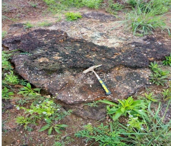
Figure 17: Highly ferruginized sandstone unit
