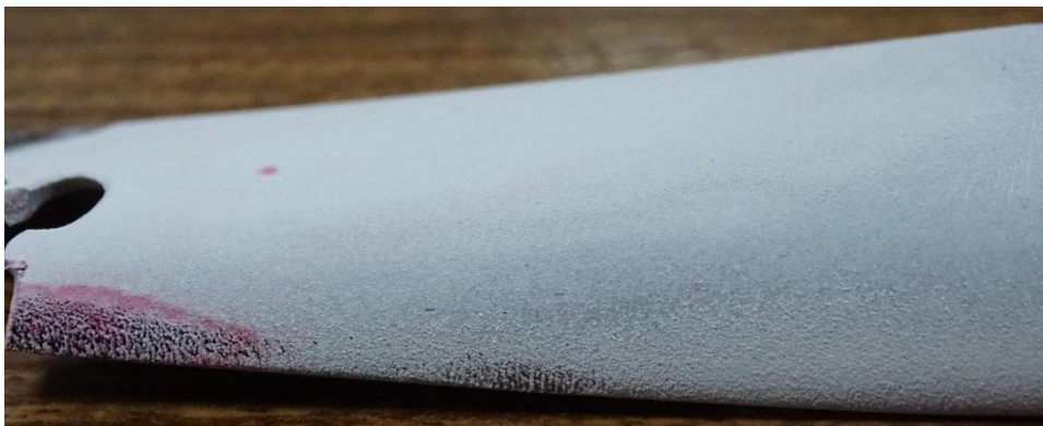
Figure (4) penetration test show no further cracks on blade.
