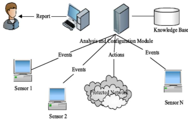
**Fig 1: Architecture of typical IDS.**
