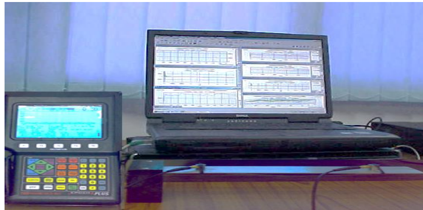
Fig. 2 Damping measurement experimental setup (EPOCH 4PLUS)
