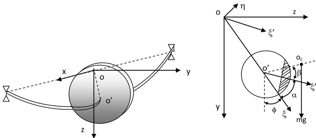
Fig.1 Geometry of crack in a Jeffcott rotor
