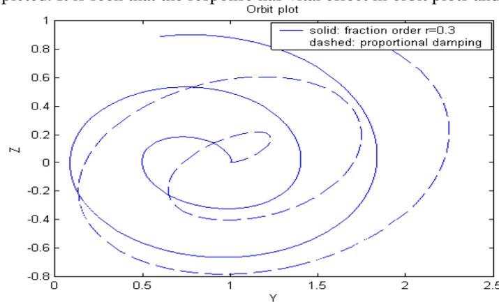
**Fig.2 Orbit plot of rotor at s=1**
