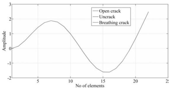
Fig.viii: Third mode of transverse vibration.
