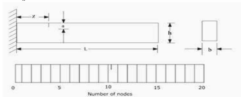
Fig. ii: Geometry of the cantilever beam with a crack.
