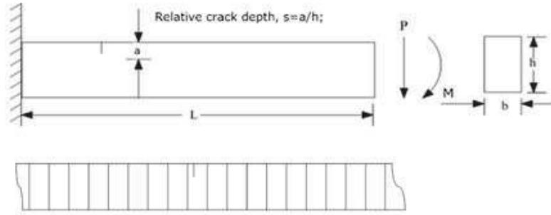
Fig. i: Schematic diagram of a beam.
