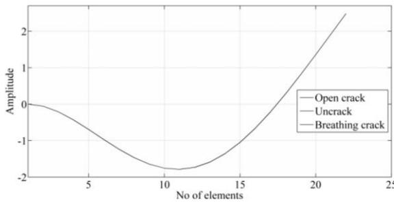
Fig. vi: Second mode of transverse vibration.
