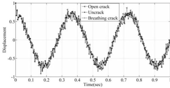
Fig. x: Comparison of the state space response of uncrack, open crack, and breathing cracked Beam.
